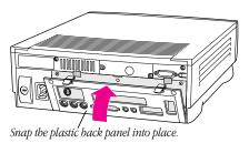
**19** Reconnect the power cord and any cables you disconnected at the start of this process.
